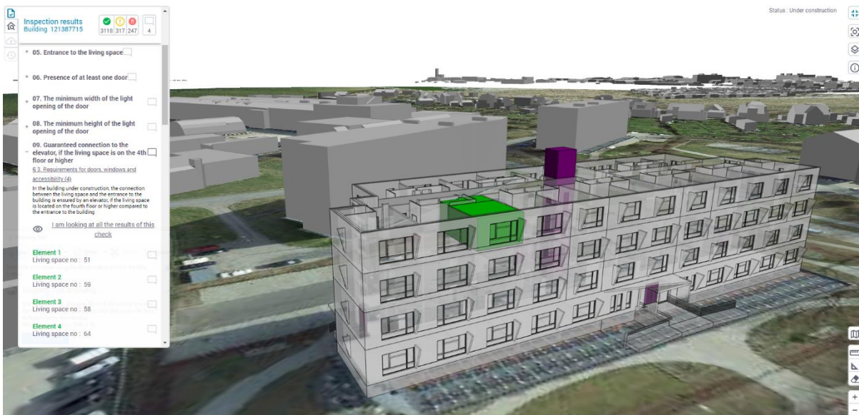
Figure 3. An IFC model with automated check results, located in its correct geographical coordinates, surrounded by layers from National Digital Twin.
