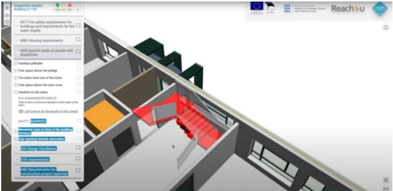
Figure 2. An example where the use of voxelisation showed that people can fall from the stair flight due to a lack of protection (railing, etc.). Source: ACCORD demo country Estonia.
