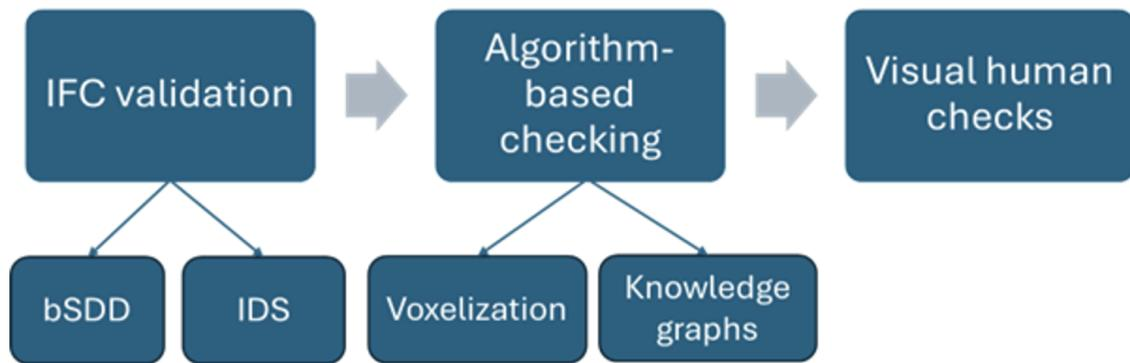
**Figure 4:** Steps (with suggested services and technologies) to improve the reliability of IFC files and compliance checks.
