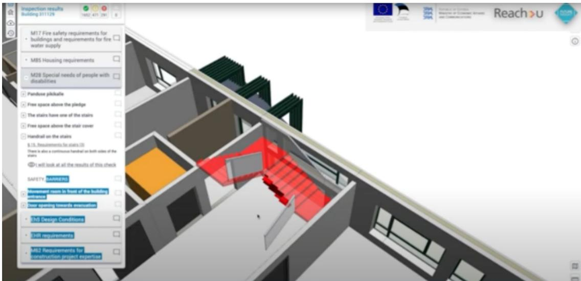
**Figure 2:** An example where the use of voxelisation showed that people can fall from the stair flight due to a lack of protection (railing, etc). Source: ACCORD demo country Estonia
